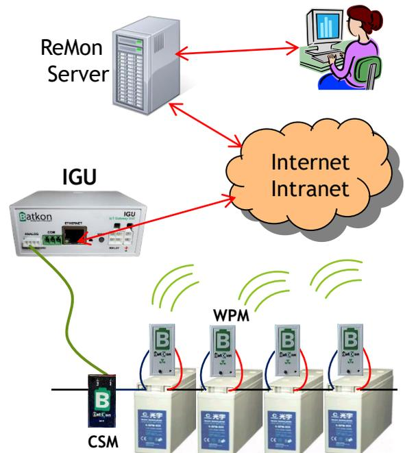
Communication with UPS / Rectifier systems can be provided over MODBUS-Serial protocol with RS-485 interface. In this way, in case of any battery reaching an overcharge voltage, it can inform the charging system about the reduction or interruption of the charging current. It can also transmit information to the power system to stop the discharge in case of over-discharge.
