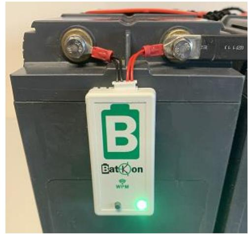
CSM module can measure charge/discharge current up to 100A bi-directionally. Hall Effect current sensors can also be connected to the IGU in higher current applications. In this way, the system can even measure currents of thousands of Amperes.
